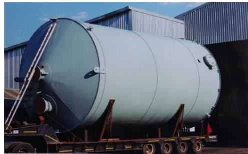
Main Surface Fan Ducting (5.2m Dia x 12m long)
