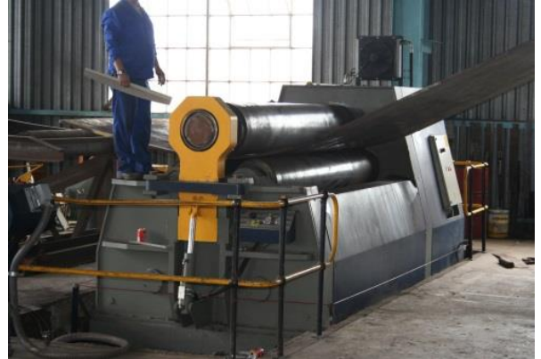
Plate Roll Capacity: 35mm x 3m wide
