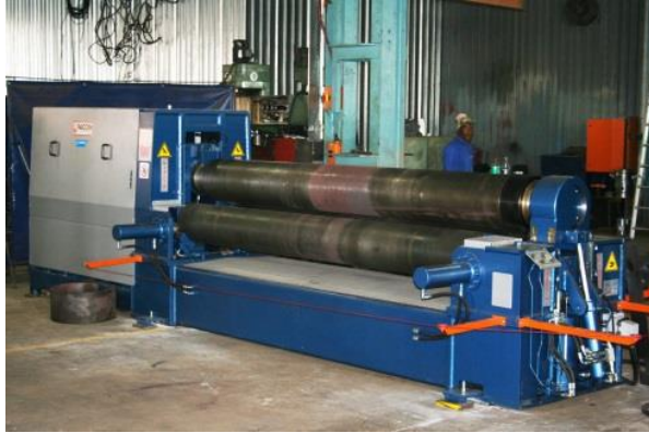
Plate Roll Capacity: 25mm x 3m Wide
