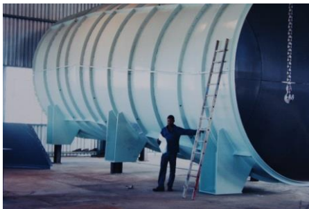
Main Surface Fan Ducting (5.2m Dia x 12m long)
