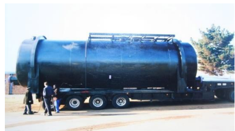
Sulphur Storage tank (3.8m dia x 12.3 m long)
